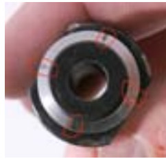
Marks on the end of a pull stud that is either not correct for the machine spindle gripper, or the gripper is damaged.
