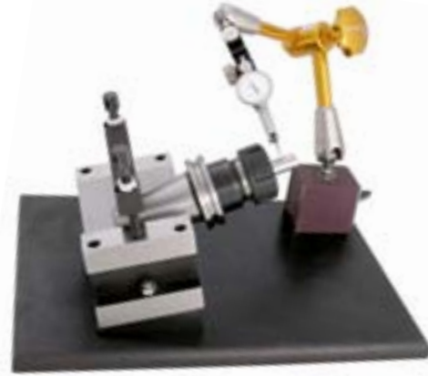
Regular bench checking of collet and nut toolholder assemblies using a gauge pin will quickly identify any T.I.R. issues.
